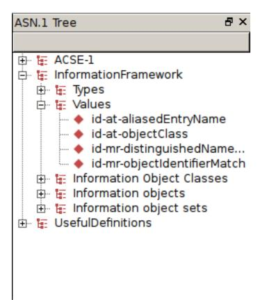
Once a schema has been validated or compiled in ACGUI, the ASN.1 Tree window provides an interactive view of the ASN.1 types defined in it. At the top level of the tree, the modules of the schema are shown. Each of these modules can be expanded to reveal branches for the types, values, information objects, etc. defined in each of them. Clicking on any node of the tree will show the relevant ASN.1 definition in a built-in browser in the editor window.
