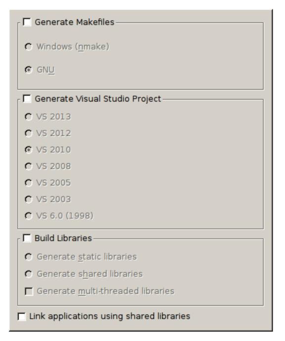
For C and C++, a makefile can be generated in either Windows or GNU format. For Windows, a Visual Studio project can also be generated. Under "Build Libraries", which will generate the build script to build a library rather than an executable, the desired variety of library can be selected.
