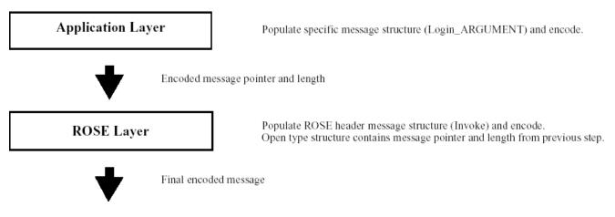
On the decode side, the process would be reversed with the message flowing up the stack:
