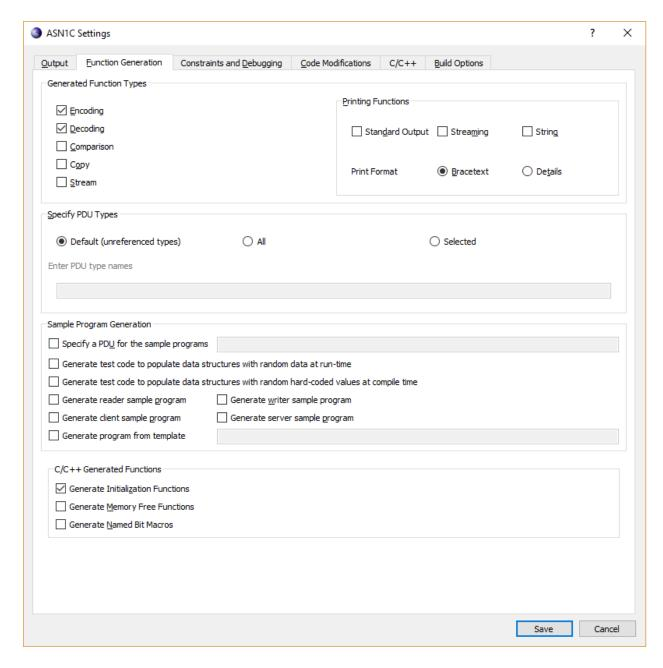
The "Function Generation" tab provides settings for what functionality to include in generated code. Options under "Generated Function Types" provide granular control of what functions to generate. The printing functions allow for various printing schemes to be generated, such as print-to-string and print-to-standard-output, and how the printed data should be formatted.
