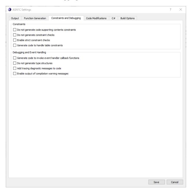
The "Constraints and Debugging" tab holds settings related to constraint handling, event handling, and logging in generated code. Under "Constraints", various types of constraint checks can be added or removed from generated code.
