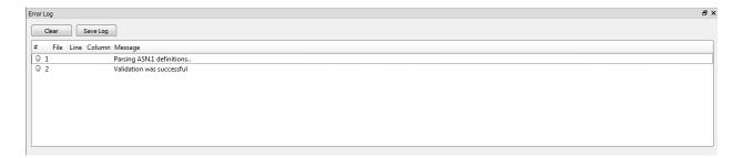
The Error Log window displays messages related to schema validation and compilation. Whenever a schema is successfully validated or compiled, the Error Log will report a success. If an error occurs, an error message will be displayed.
