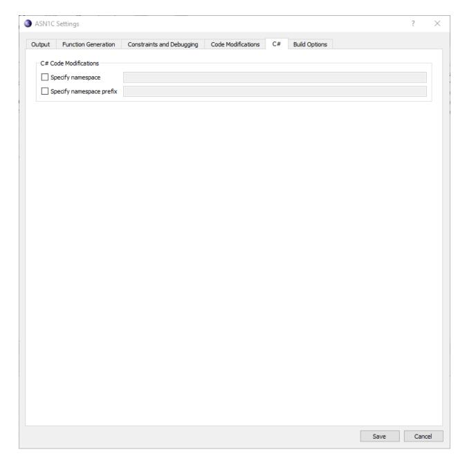
In this, modifications allow for manipulating the namespace into which code is generated. The Java tab contains similar options.
