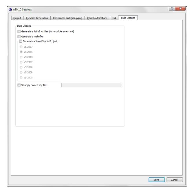
Similarly for C#, a makefile or Visual Studio project can be created, optionally including a \*.mk file listing the files generated. An option to specify a strongly named key file also exists.
