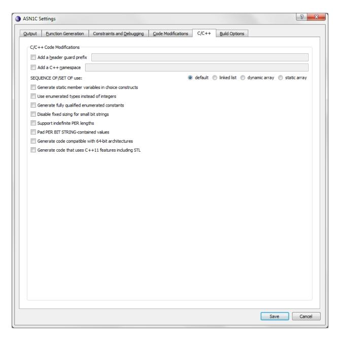
In this case, code modifications include several settings for adjusting how ASN.1 types are mapped to native C/C+ + types.
