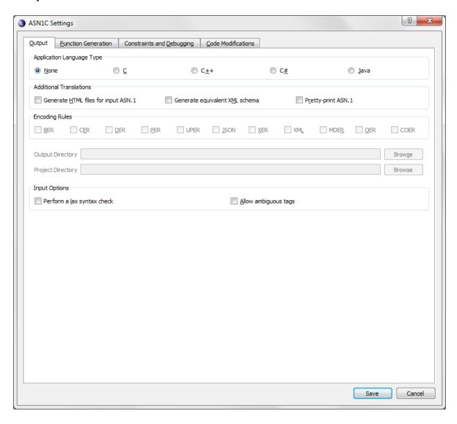
The "Output" tab contains options for selecting a target language, encoding rules, output directory. In order to compile a schema, a target language must be selected under "Application Language Type".
