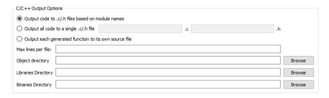
For C or C++ target languages, "C/C++ Output Options" controls how generated code is distributed across source files.
