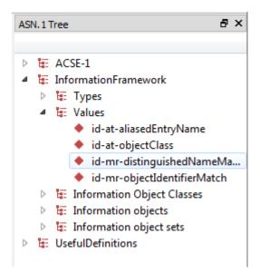
Once a schema has been validated or compiled in ACGUI, the ASN.1 Tree window provides an interactive view of the ASN.1 types defined in it. At the top level of the tree, the modules of the schema are shown. Each of these modules can be expanded to reveal branches for the types, values, information objects, etc. defined in each of them. Clicking on any node of the tree will show the relevant ASN.1 definition in a built-in browser in the editor window.
